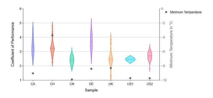
Range of coefficient of performance when outside temperature is between -10 and 5°C. Credit: *Joule* (2023). DOI: 10.1016/j.joule.2023.08.005
