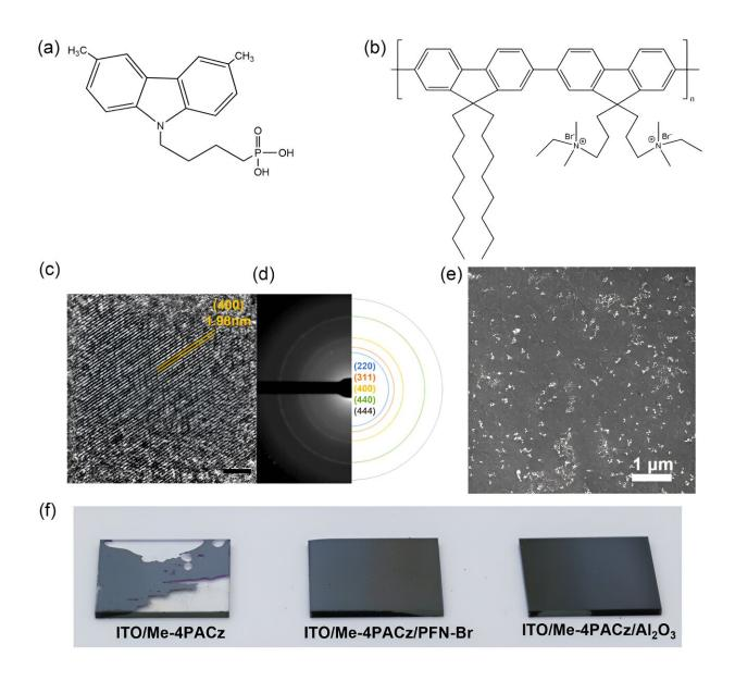
Molecular structure of a) Me-4PACz and b) PFN-Br. c) A high-resolution TEM and d) the related SAED pattern of the Al<sub>2</sub>O<sub>3</sub> NPs used in this study. e) Scanning
