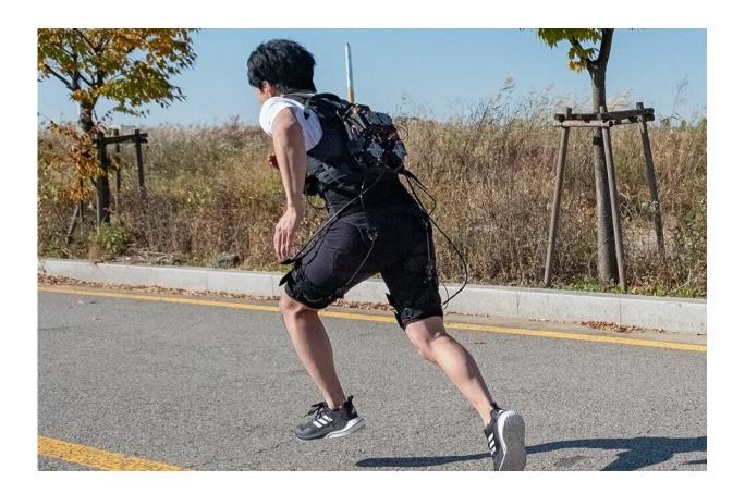
The exosuit is made of textile garments at the waist and thighs, and an actuation system with high control bandwidth performance to the back side. It showed the first reduction of the sprint time in the real world to the non-elite runners. Credit: Assistive and Rehabilitation Robotics Lab at Chung-Ang University
