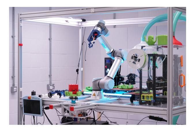
The ARE Robot Fabricator (RoboFab). Evolved robot skeletons (green) are 3D printed, the robot arm equips them with a central 'head' (red) and then attaches modular 'organs' (dark blue) to the skeleton. Spring-loaded clips enable the mechanical connections, and wires connect the organ electronics to the 'head' to provide power and control signals. All aspects of this process: 3D printing, assembly, interconnections and electronics, impose their own constraints on the
