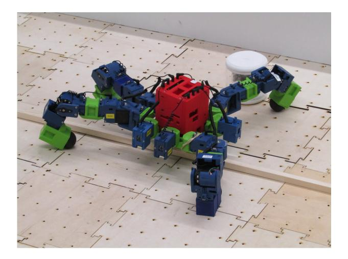
An evolved robot with legs and sensors. The viability of such body plans is strongly determined by the capabilities of the underlying electronic system. Credit: Angus et al.
