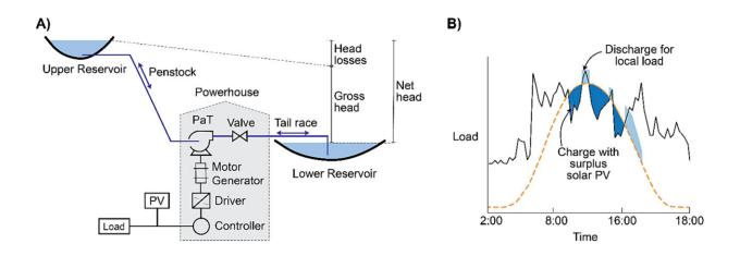
A) Hardware configuration for micro-PHES B) Example charge-discharge operation for micro-PHES adapted Morabito and Hendrick noting that solar generation capacity (kW), storage capacity (kW, kWh) and load will alter the charge and discharge profiles. Credit: *Applied Energy* (2023). DOI: 10.1016/j.apenergy.2023.121715
