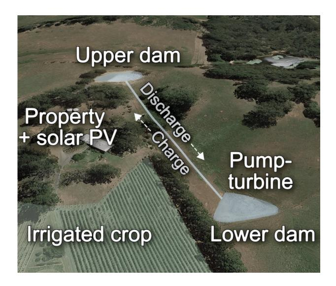
Micro-pumped hydro energy storage systems store excess solar energy from high-
