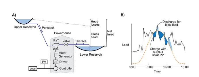
A) Hardware configuration for micro-PHES B) Example charge-discharge operation for micro-PHES adapted Morabito and Hendrick noting that solar generation capacity (kW), storage capacity (kW, kWh) and load will alter the charge and discharge profiles. Credit: *Applied Energy* (2023). DOI: 10.1016/j.apenergy.2023.121715
