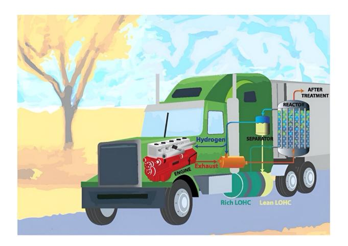
An MIT team has modified a transport truck's powertrain to allow onboard hydrogen release from the liquid organic hydrogen carriers. Credit: The Green Group
