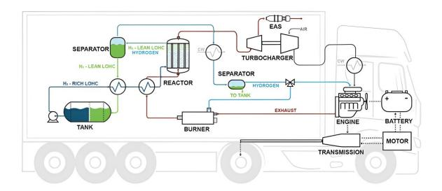
Proposed process flow diagram for onboard dehydrogenation. Component sizes are not to scale and have been enlarged for illustrative purposes. Credit: The Green Group
