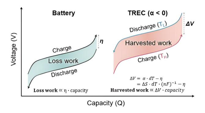
Schematic showing the different mechanisms of a battery and TREC system. Credit: UNIST
