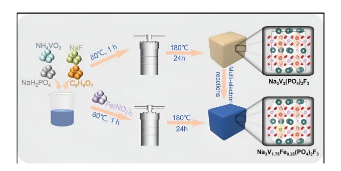
Schematic of NVFePF material synthesis. Credit: *Energy Material Advances* (2023). DOI: 10.34133/energymatadv.0050
