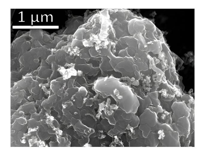
Scanning electron microscope (SEM) image of layered stacks of nano-scale flash graphene sheets formed from waste plastic. Credit: Kevin Wyss/Tour lab
