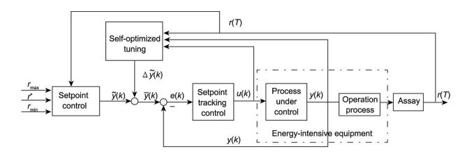
Structure of the intelligent control method for low-carbon operation. Credit: Tianyou Chai et al.
