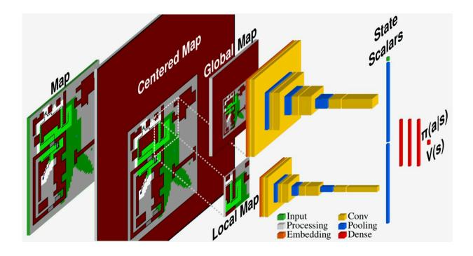
How the reinforcement learning agent observes and processes the environment. It observes a map representation of the problem, which it then centers around its position. It then compresses the entire centered map into a global map with reduced resolution and a full-resolution local map, which shows only the immediate vicinity of the agent. The agent then processes these two maps through different neural network layers until the agent outputs an action decision. Credit: Theile et al.
