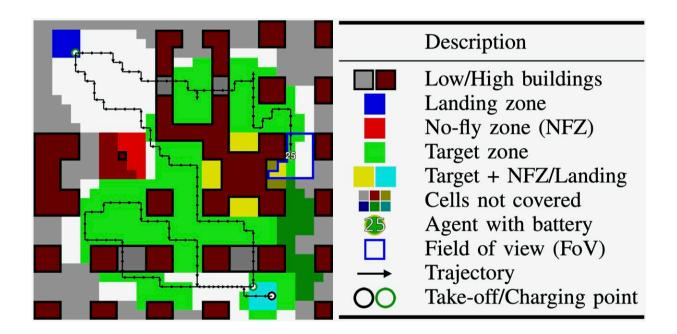
The coverage path planning scenario in which the agent needs to find a trajectory that covers all of the green areas with its field of view without flying into obstacles and with recharging in blue landing zones. Credit: Theile et al.
