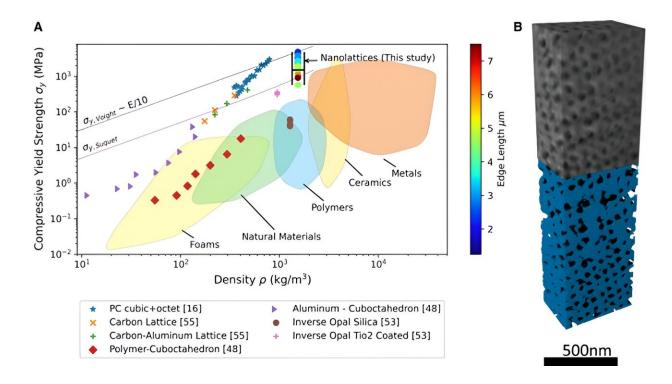
A graph comparing the nanolattice in this experiment to the relative strength of various materials. Credit: Brookhaven National Laboratory
