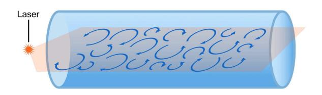
A sheet of laser light is being shone through the clear pipe through which water is pumped continuously. The laser gets reflected by tiny particles in the water and makes its swirling currents visible. Credit: © Thomas Zauner / ISTA
