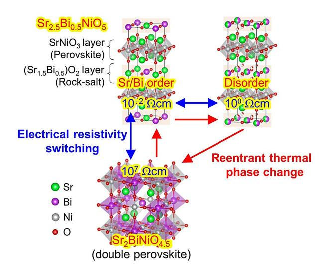
Schematics of electrical resistivity switching and reentrant thermal in
