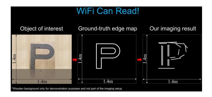
Sample imaging in non-through-wall settings: Their method can image details of letter P in ways not possible before. Credit: Mostofi Lab
