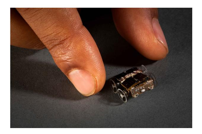
Researchers at the University of Washington have created MilliMobile, a tiny, self-driving robot powered only by surrounding light or radio waves. It's about the size of a penny and can run indefinitely on harvested energy. Credit: Mark Stone/University of Washington
