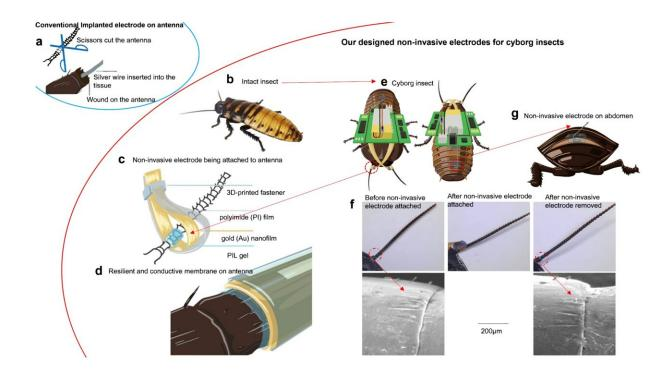
Non-invasive electrodes with resilient and conductive membrane for cyborg insects. Credit: *npj Flexible Electronics* (2023). DOI: 10.1038/s41528-023-00274-z
