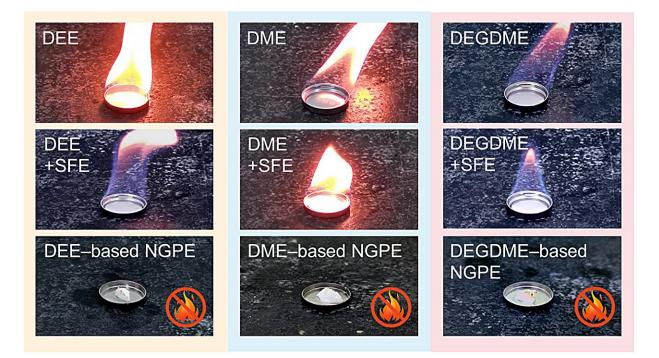
Non-flammable quasi-solid-state gel electrolyte to eliminate safety hazard for high-energy lithium metal batteries. Credit: Meng et al.
