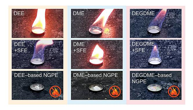
Non-flammable quasi-solid-state gel electrolyte to eliminate safety hazard for high-energy lithium metal batteries. Credit: Meng et al.
