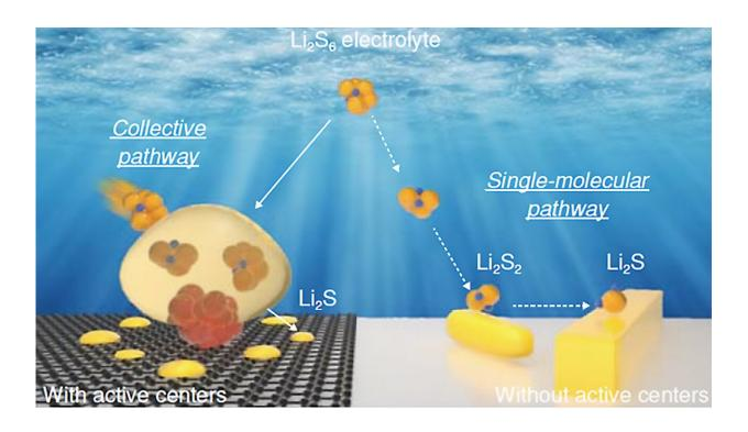
Different reaction pathways from lithium polysulfide ( $\text{Li}_2S_6$ ) to lithium sulfide ( $\text{Li}_2S$ ) in lithium-sulfur batteries with (left) and without (right) catalyst in sulfur cathode. Credit: Argonne National Laboratory
