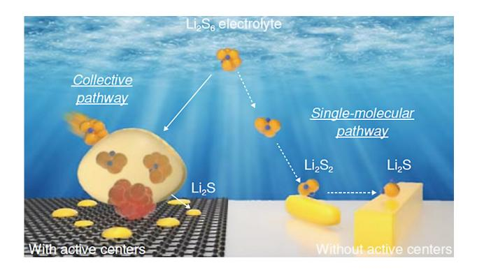
Different reaction pathways from lithium polysulfide  $(Li_2S_6)$  to lithium sulfide  $(Li_2S)$  in lithium-sulfur batteries with (left) and without (right) catalyst in sulfur cathode. Credit: Argonne National Laboratory
