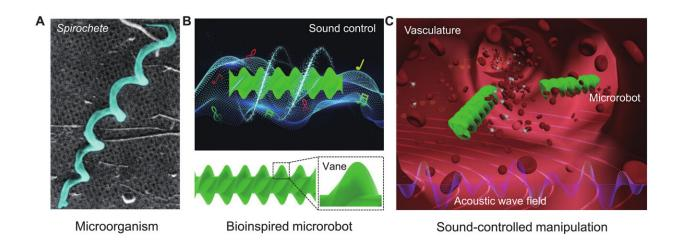
Spirochete-inspired propulsion based on acoustic actuation.(**A**) Micrograph showing the spiral morphology of *Spirochete* bacteria, which execute translation motion through rotation in viscosity-dominated fluids. (**B**) An illustration of a wireless bioinspired robot that propels in response to an external sound field. (**C**) A concept schematic illustrates the use of such microrobots for noninvasive surgery in vasculatures. Credit: *Science Advances* (2023). DOI: 10.1126/sciady.adh5260
