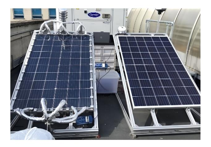
Solar PV-T collector panels on a roof at Imperial College. Credit: Imperial College London
