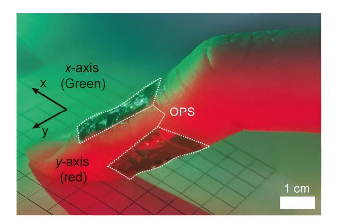
Photograph of organic light-responsive sensors attached to the top (x-axis) and side (y-axis) of the index finger on a graph paper of 25 cm<sup>2</sup>. Credit: Cho et al, *Nature Electronics* (2023). DOI: 10.1038/s41928-023-01012-z
