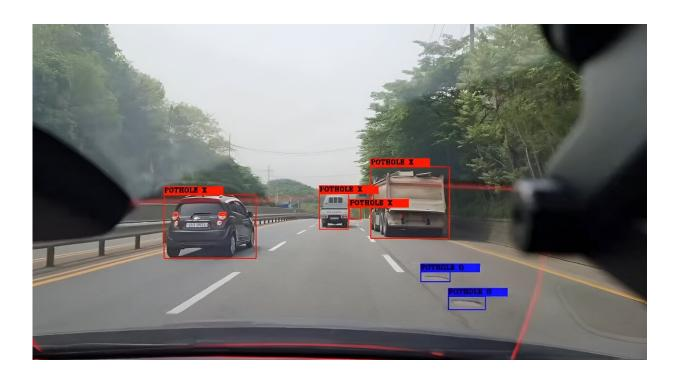
Pothole inspection screen using artificial intelligence pothole filtering program (blue: pothole correct, red: not pothole). Credit: Korea Institute of Civil Engineering and Building Technology (KICT)
