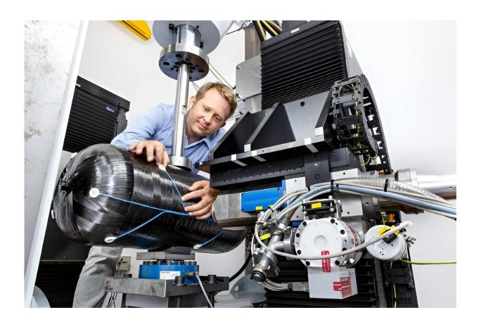
The HyMon pressure tank is damaged before use at Fraunhofer LBF. The acoustic emission sensors detect damage to the tank and provide data for calculation models. Credit: Fraunhofer LBF/Ursula Raapke
