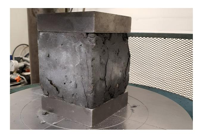
A block of concrete made with waste foundry sand. Credit: Nottingham Trent University
