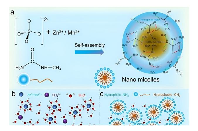
Schematic diagram of nanomicellar electrolyte. Credit: University of Science and Technology of China
