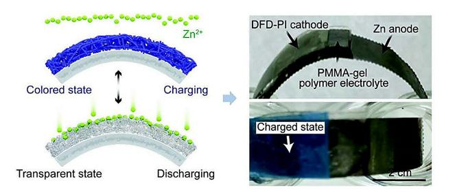
Electrochromic zinc ion battery whose anode is made of a polymer that turns dark blue when charged and transparent when discharged. Credit: *Advanced Materials* (2023). DOI: 10.1002/adma.202301141
