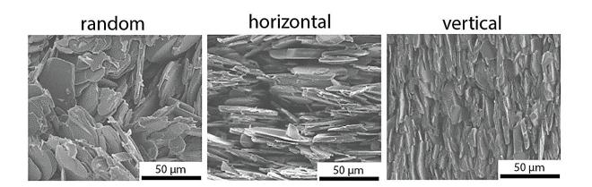
Microscopic particles of hexagonal boron nitride in various configurations. Credit: Nanyang Technological University
