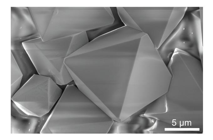
Scanning electron microscope image of six-element single crystals. The crystals are formed from building blocks of "multielement ink," the first high-entropy semiconductor that can be processed at low-temperature or room temperature. Credit: Maria Folgueras and Peidong Yang/Berkeley Lab/Nature.
