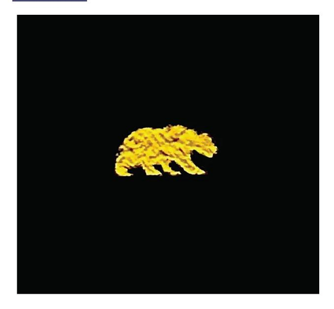
Photoluminescent image of the California Golden Bears logo emitted from fiveelement ZrSnTeHfPt single crystals under UV lamp excitation. The crystals were formed from "multielement ink." The experiment demonstrates the material's potential as a color-tunable LED device. Credit: Maria Folgueras and Peidong Yang/Berkeley Lab
