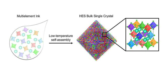
In solution, multielement ink self-assembles at low temperatures into highentropy semiconductors or halide perovskite single crystals. Credit: Maria Folgueras, Yuxin Jiang, and Peidong Yang/Berkeley Lab/Nature.
