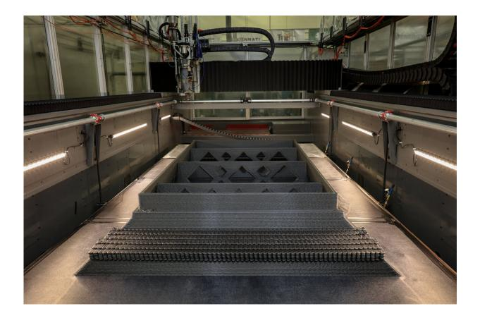
ORNL's 3D-printed polymer composite mold was used to produce precast concrete parts for a New York City building. Researchers conducted a technoeconomic analysis that highlights the benefits over wood molds. Credit: ORNL, U.S. Dept. of Energy and Gate Precast
