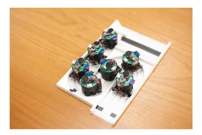
A team led by researchers at the University of Washington has developed a shape-changing smart speaker, which uses self-deploying microphones to divide rooms into speech zones and track the position of individual speakers. Here, the swarm of robots is shown in its charging station, which the robots can return to automatically. Credit: April Hong/University of Washington
