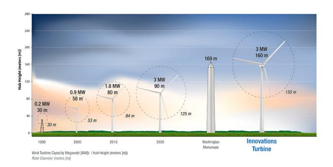
Wind turbines have been increasing in tower (or hub) height (from 30 meters [m] to 90 m) and rotor diameter (from 30 m to 125 m) from the 1990s to the 2020s, with power capacity also growing from 0.2 megawatts (MW) to 3 MW. Near-commercial innovations can produce turbines with tip heights taller than the top of the Washington Monument (169 m tall) when a rotor with a 150-m diameter is attached to a 160-m tower. Credit: Josh Bauer, NREL
