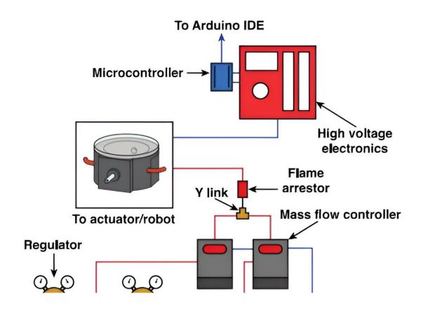
Block diagram of the microactuator and microrobot testing apparatus. Two gas cylinders supply the reactant gases. Flow and mixing is regulated by offboard mass flow controllers. Ignition is achieved via high voltage, spark-generating electronics that are controlled via an Arduino. Credit: *Science* (2023). DOI: 10.1126/science.adg5067. https://www.science.org/doi/10.1126/science.adg5067
