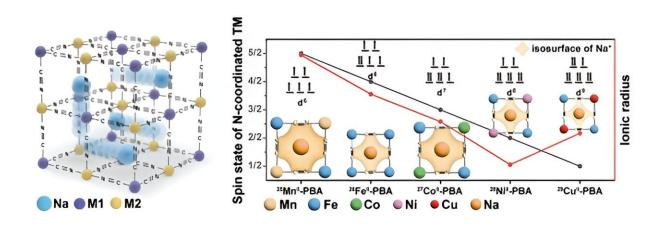
(a) Schematic illustration of PBA framework and the Na<sup>+</sup> diffusion path. b) Correlation between the spin state of N-coordinated transition metal ions and their lattice parameters. Credit: Ulsan National Institute of Science and Technology
