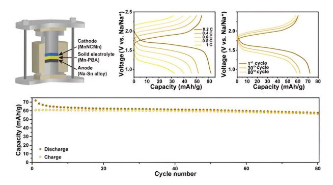
From top right are the schematic illustration of MnNCMn/SE/Na<sub>3</sub>Sn ASNBs using Mn-PBA as the SE, and the rate performance and charge–discharge voltage profile of the ASNBs at 30°C as functions of the C-rates and number of cycles. On the bottom is the cycle performance of the ASNBs at a current density of 0.2C-rate and 30°C. Credit: Ulsan National Institute of Science and Technology
