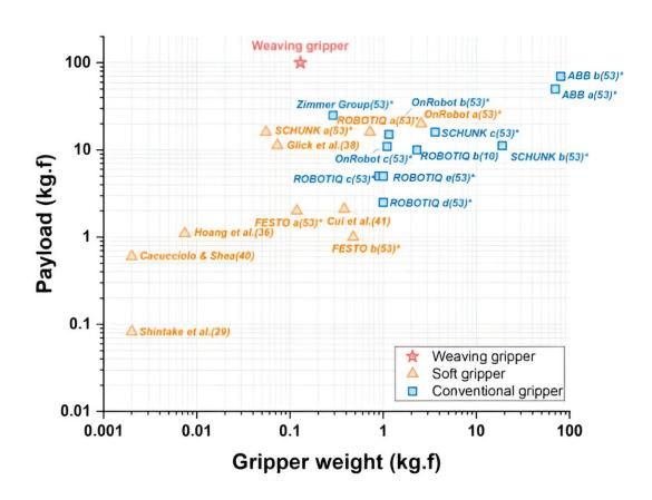
Comparison of gripper weight to payload (maximum weight the robot can lift) for the woven gripper, soft gripper, and rigid gripper. Credit: Korea Institute of
