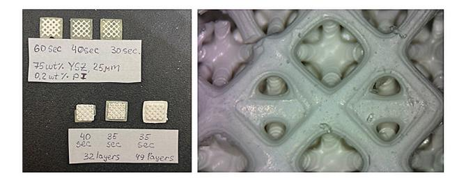
The researchers optimized the 3D printing process by varying such parameters as printing layer thickness and sintering time. Credit: Igor Pchelintsev
