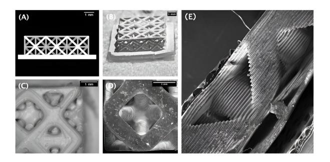
Model (A) and photos of the ceramic structure 3D-printed by Skoltech researchers. It could improve the efficiency of fuel cells, a promising technology for cleaner fossil fuel consumption. Credit: Igor Pchelintsev
