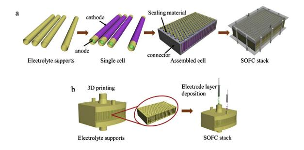
Fuel cells manufactured conventionally (a) and with 3D printing (b). Credit: Igor Pchelintsev
