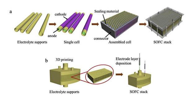
Fuel cells manufactured conventionally (a) and with 3D printing (b). Credit: Igor Pchelintsev
