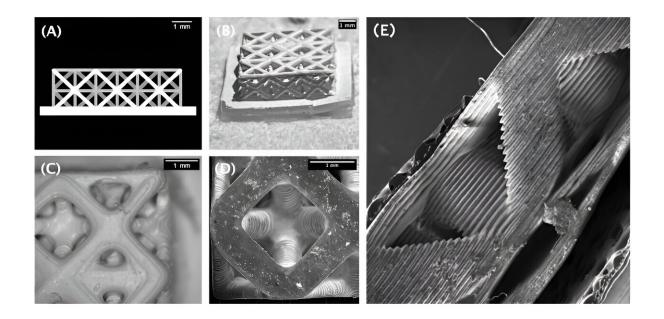
Model (A) and photos of the ceramic structure 3D-printed by Skoltech researchers. It could improve the efficiency of fuel cells, a promising technology for cleaner fossil fuel consumption. Credit: Igor Pchelintsev
