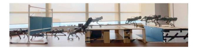
A timelapse photo showing how the dog-like robot is able to navigate a variety of obstacles autonomously. Credit: Shanghai Qi Zhi Institute/Stanford University
