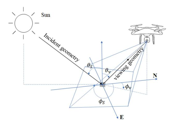
Schematic diagram of bidirectional reflection elements. Credit: *Remote Sensing* (2023). DOI: 10.3390/rs15205000
