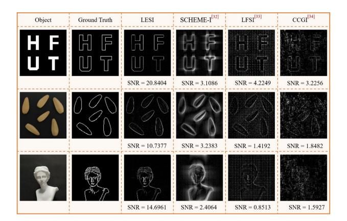
The performance of the LESI method proposed in this study was compared with that of recently reported edge detection schemes. (ESI: edge-sensitive single-pixel imaging. LESI: ESI with Laplacian operator). Credit: *Intelligent Computing* (2023). DOI: 10.34133/icomputing.0050
