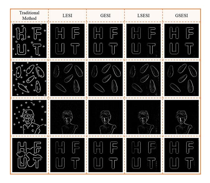
In the presence of light pollution from a green laser (top three rows) and white LED (bottom row), the traditional edge detection method yields many false edges, whereas all four variants of the new method detect only the target object edges. Credit: *Intelligent Computing* (2023). DOI: 10.34133/icomputing.0050
