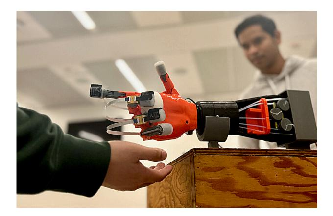
The sensor enables a prosthetic or robotic arm to respond to tactile stimuli with dexterity and precision, such as holding fragile objects like an egg without
