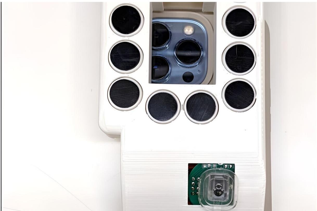
Autoclickers on the bottom of Brushlens tap the screen for users, which helps people with tremors and spasms tap their desired option on the screen. A window in the center of the case allows the phone's camera to view the items on the touchscreen menu. Credit: Chen Liang, doctoral student, Computer Science and Engineering, University of Michigan
