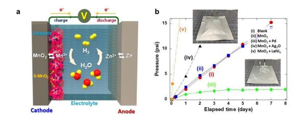
Proposed strategy for securing safety of the aqueous rechargeable batteries via water-regeneration. Credit: Korea Institute of Science and Technology
