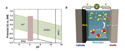
Causes of hydrogen generation and incessant accumulation within the cell in the aqueous rechargeable batteries. Credit: Korea Institute of Science and Technology
