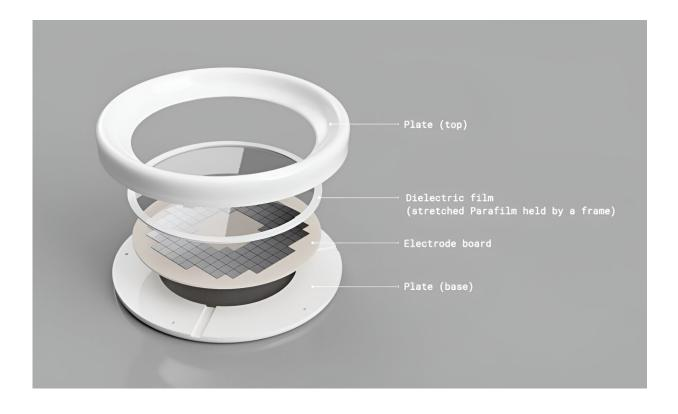
We designed a new plate that embeds "electrowetting on dielectric" technology in order to be able to execute precise motion operations of aqueous droplets. This technology utilizes electrical voltage to unbalance the force equilibrium at the solid-liquid-vapor interface, causing the droplets to move toward the charged electrodes. Credit: Monash University
