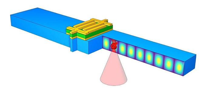
A piezoelectric layer (green) sandwiched between two electrodes (yellow) atop of a silicon carbide acoustic resonator (blue). Acoustic waves generated by the electrodes and piezoelectric layer put mechanical strain on the lattice, which flip the spin of the defect (red). The spin is read out with a laser focused onto the backside of the resonator. Credit: Hu Group/Harvard SEAS
