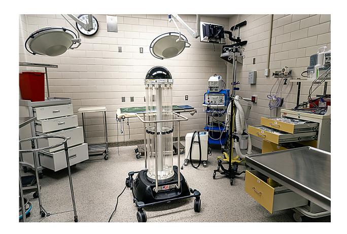
Once Trudy has been placed in a room, its 360-degree sensors determine how large the space is and how long the disinfection cycle should be. Credit: Jason Nitsch/Texas A&M University Division of Marketing and Communications
