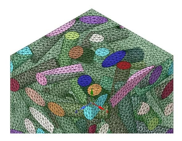
Representative volume elements with corresponding fiber distribution are used as a micromechanical model in order to estimate in situ composite properties. Credit: Fraunhofer-Gesellschaft
