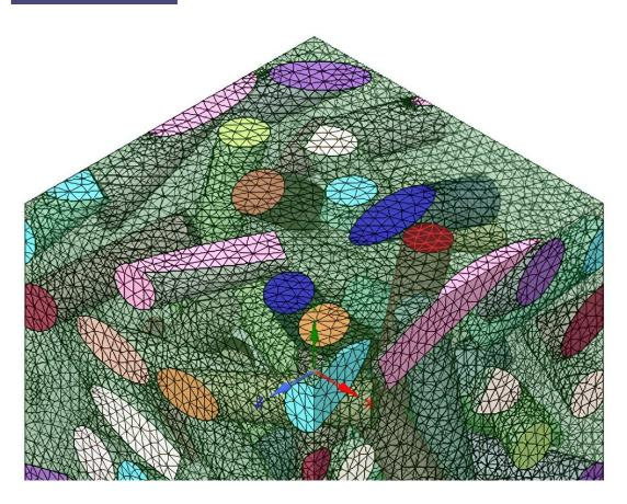
Representative volume elements with corresponding fiber distribution are used as a micromechanical model in order to estimate in situ composite properties. Credit: Fraunhofer-Gesellschaft
