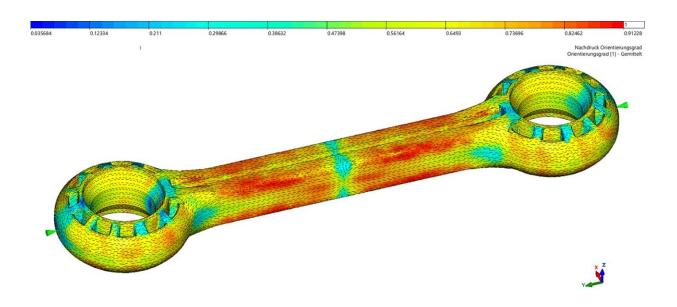
The filling simulation can provide information on the fiber orientation in the com-ponent, which affects the load distribution and strength. Credit: Fraunhofer-Gesellschaft
