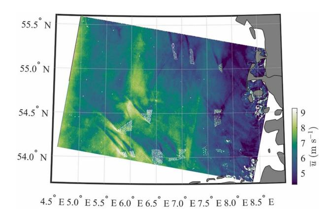
Mean wind speed u at 10 m above the sea surface observed in the German Bight by the Sentinel-1A satellite on 2022-04-17. Farm-induced wakes spanning dozen of kilometers are visible as darker areas downstream of wind turbines, which are visible as white dots. Credit: *Marine Policy* (2023). DOI: 10.1016/j.marpol.2023.105897
