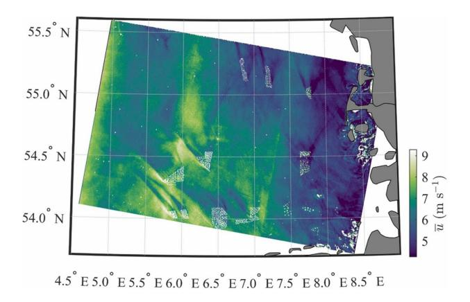
Mean wind speed u at 10 m above the sea surface observed in the German Bight by the Sentinel-1A satellite on 2022-04-17. Farm-induced wakes spanning dozen of kilometers are visible as darker areas downstream of wind turbines, which are visible as white dots. Credit: *Marine Policy* (2023). DOI: 10.1016/j.marpol.2023.105897
