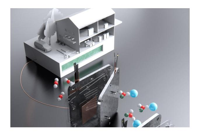
A schematic shows the formate process. The top left shows a household powered by the direct formate fuel cell, with formate fuel stored in the underground tank. In the middle, the fuel cell that harnesses formate to supply electricity is shown. On the lower right is the electrolyzer that converts bicarbonate into formate. Credit: Shuhan Miao, Harvard Graduate School of Design
