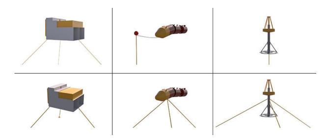
Although wave energy devices come in many shapes and sizes, most come in one of the three flavors pictured here: oscillating water column (left), attenuator (middle), and point absorber (right). For their mooring study, the researchers identified generic systems that could serve all three. Credit: Josh Bauer, NREL
