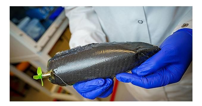
This miniature boat is built from a structural supercapacitor—a material that provides both structural support and energy storage capabilities. Credit: UC San Diego Jacobs School of Engineering
